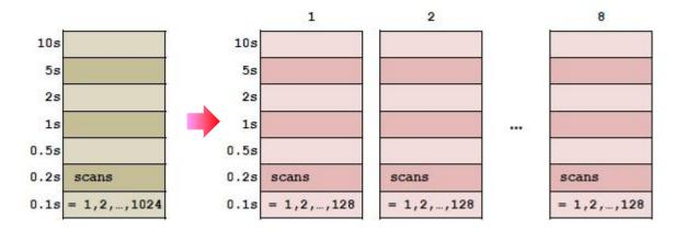
To carry out the "external scan", you can add the parameter "outer\_scans" in Acquisition tab. In the above example, input 8 as outer\_scans as well as 128 as scans. To save the data after every set of the acquisition, you can use mod\_save. Here, please be cautious in setting the value of mod\_save as the number of one set acquisition, namely, the multiple of 7 (0.1,0.2,...,10s) by 128 scans equal to 896.
