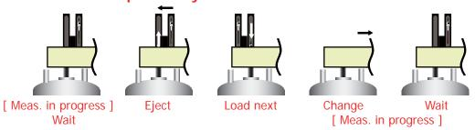
In tandem manipulator system, a succeeding sample is conveyed to wait at the top of the magnet during NMR measurements, and to load the sample at finish time the slot moves only 10cm. Thus, almost all the motions are executed during measurements, saving total experimetal time.
