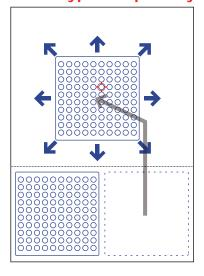
A 10 x 10 matrix sample tray moves freely in the x and y directions and so quickly changes samples located far apart.
