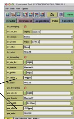
Fig. 4 Parameter setting window for ^{19}\text{F} double irradiation.
