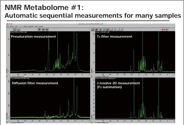
**Results of full automatic measurements for human blood serum** All the measurements, incorporating solvent signal suppression, are automatically set up and accomplished.
